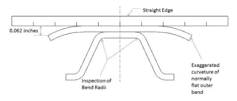
Figure 1 to paragraphs (k)(1)(iii) and (v) of this AD: Cross section of v-band coupling
