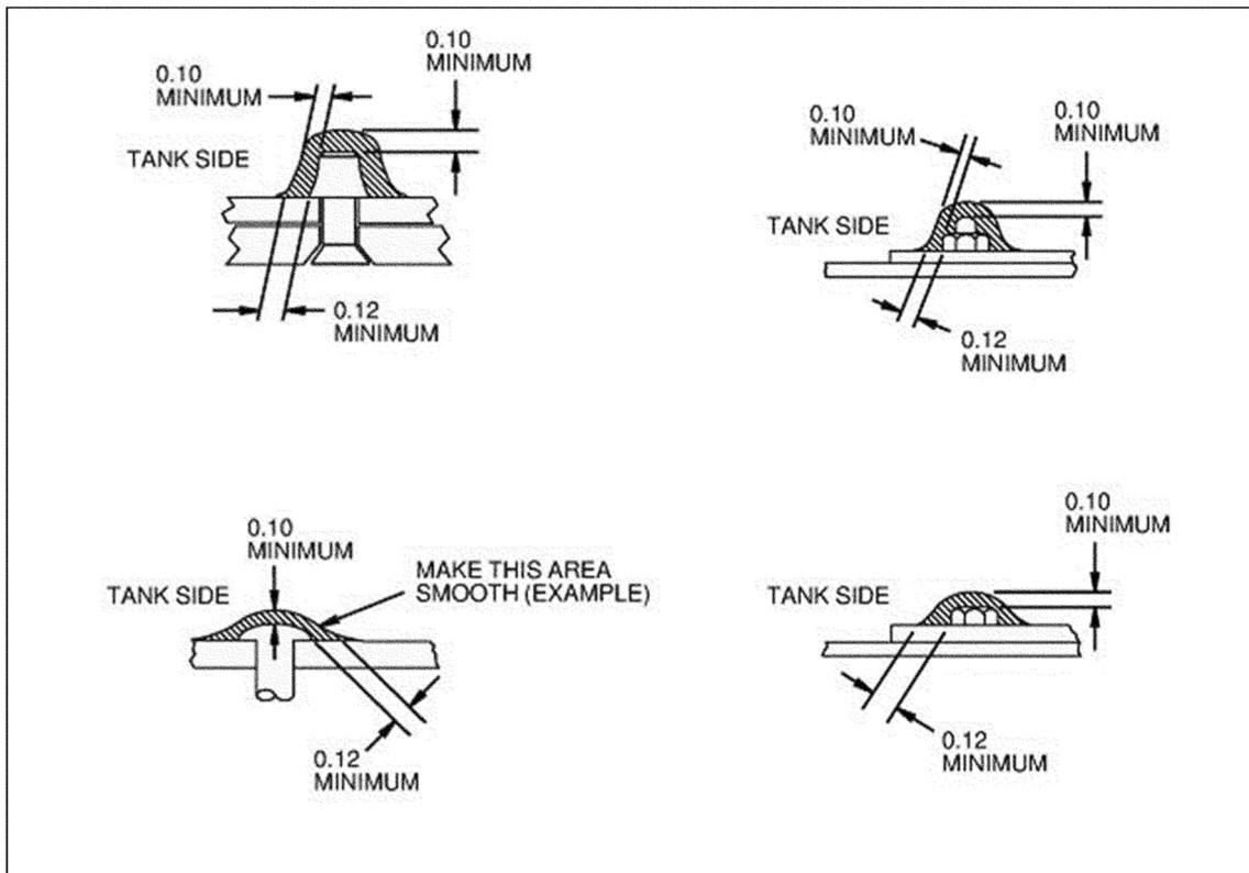
(4) Where Boeing Alert Requirements Bulletin 777-53A0100 RB, dated March 16, 2023, specifies doing actions “in accordance with Revision 2 of Boeing Service Bulletin 777-53-0084,” for this AD, where flagnote (f) of Figure 7 and Figure 22 of that referenced service information (“Revision 2 of Boeing Service Bulletin 777-53-0084”) includes a sealant callout of Boeing Material Specification (BMS) 5-45 or an optional BMS 5-95, only BMS 5-45 is allowed.
