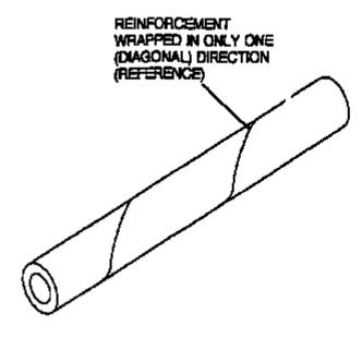
OLD STYLE 951-10 HOSE WITH REINFORCEMENT WRAPPED IN ONLY ONE (DIAGONAL) DIRECTION THE LENGTH OF THE HOSE (REMOVE AND REPLACE WITH REPLACEMENT STYLE HOSE)
