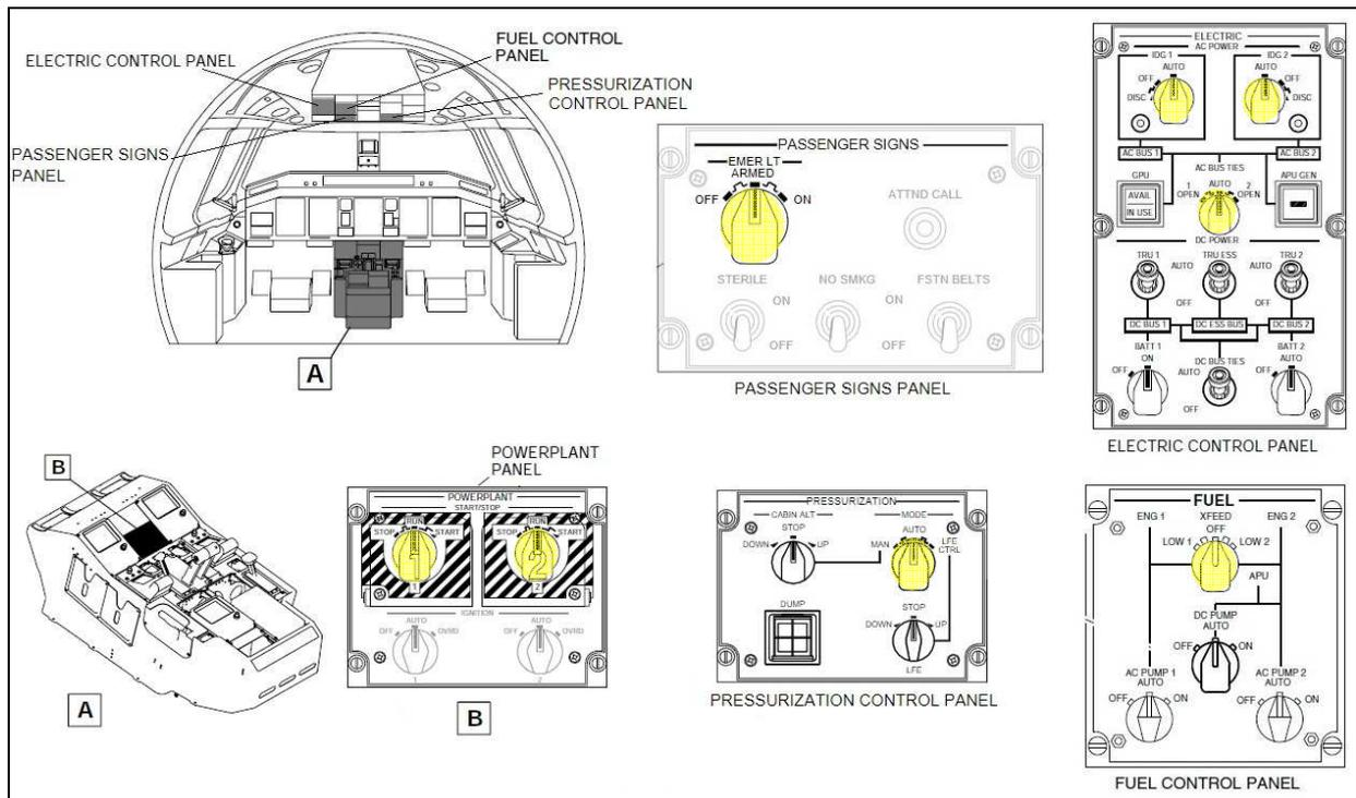
Figure 5 – ERJ-170/190 Panels (typical) – Relevant switches are highlighted
