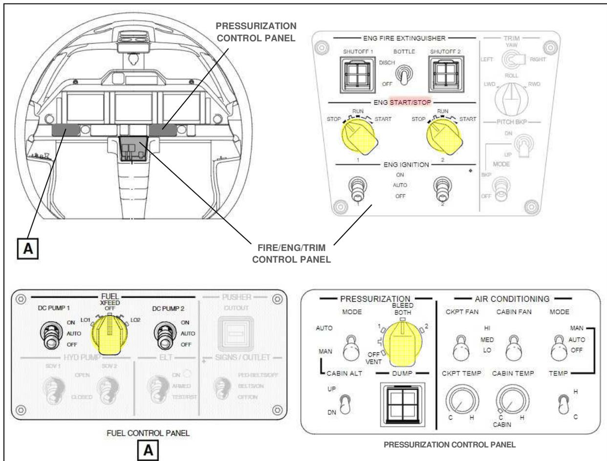
Figure 3 – EMB-500/505 Panels (typical) – Relevant switches are highlighted
