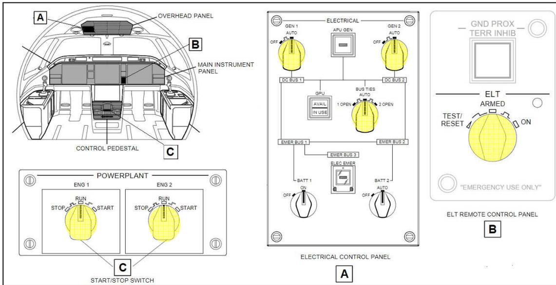
Figure 4 – EMB-545/550 Panels (typical) – Relevant switches are highlighted
