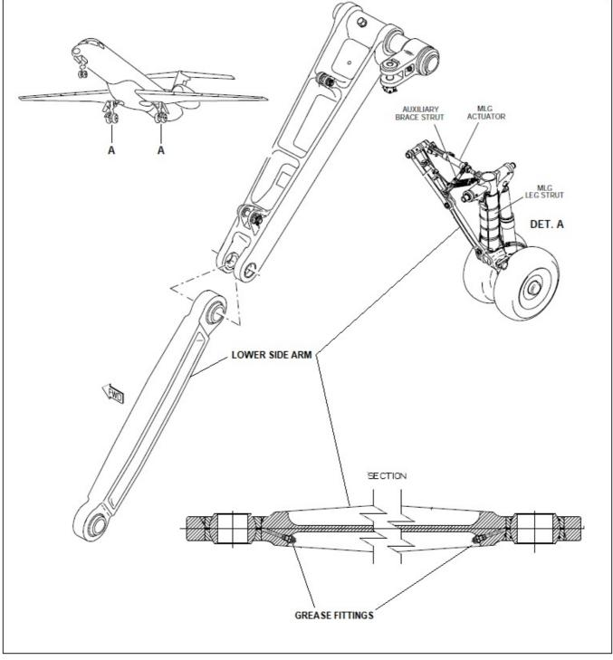
Figure 1: MLG Lower Side Arm correct grease fittings installation
