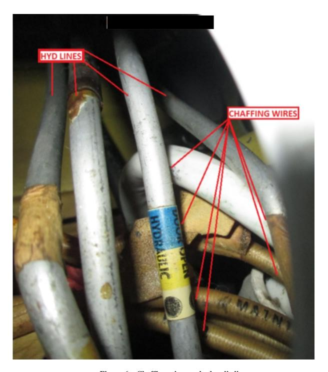
Figure 6 – Chaffing wires on hydraulic lines
