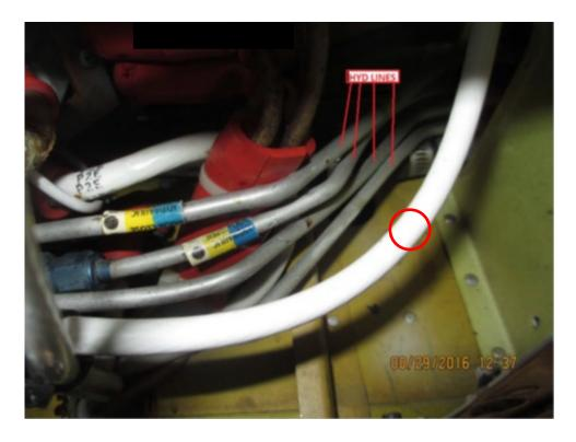
Figure 4 – View of the Hydraulic Lines in close proximity with electrical wires
