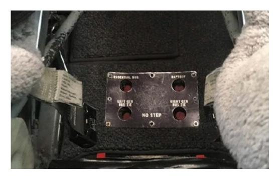
Figure 3 – Floor Mounted CB Panel – Interior (Typical of pre-1981 production)
