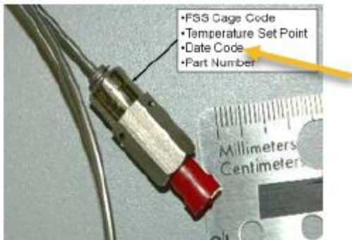
Figure 4-51. Identification Markings on Coaxial SE Female (Socket) Connector
