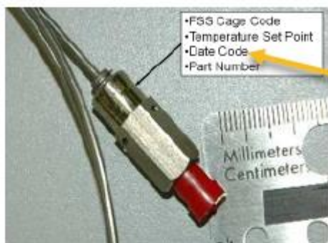
Figure 4-51. Identification Markings on Coaxial SE Female (Socket) Connector
