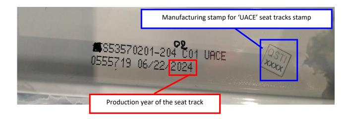
The identification of the seat track is located on the lower face of the seat track.
