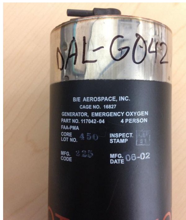
Figure 2 – MFG.DATE (06-02 = June 2002) example
