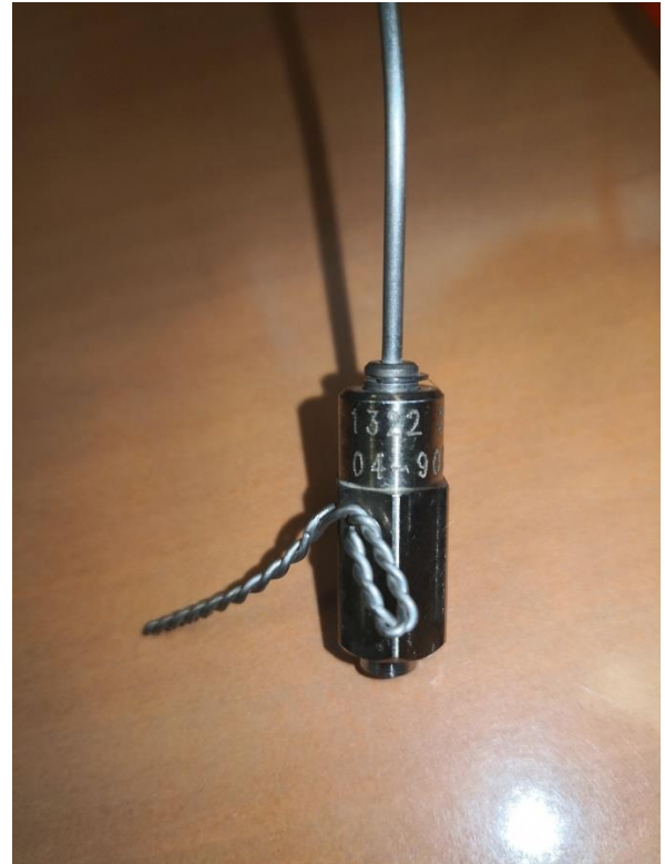
Figure 4-51. Identification Markings on Coaxial SE Female (Socket) Connector
