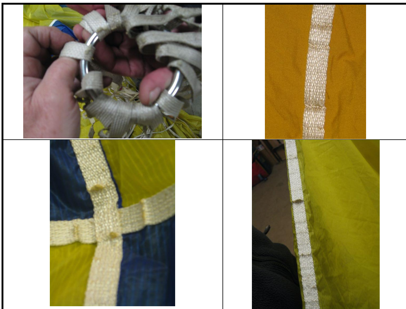
Figure 1: Examples of load tape damage
