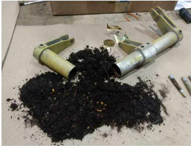
Figure 1 Corrosion on the inside of elevator torque shaft
