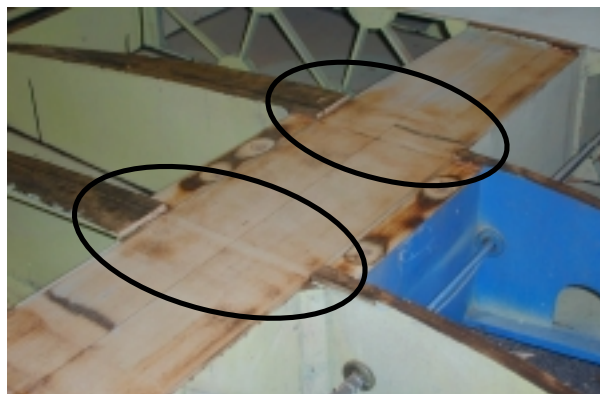
Photo 3: example of airplane with reinforcements in good condition. Therefore the only parts removed were covering the main spar.
