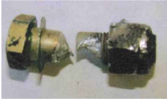
Figure 2: Corroded Earth Terminal Point
