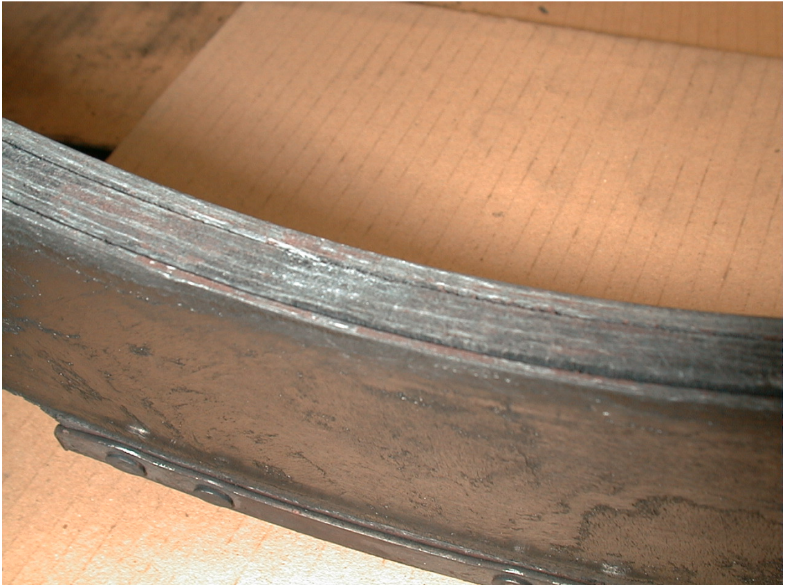
Rotor R1 – " 3 for 1" ( t=1.5 -7- 2.5 mm) + reddish Ox. Inhib.
