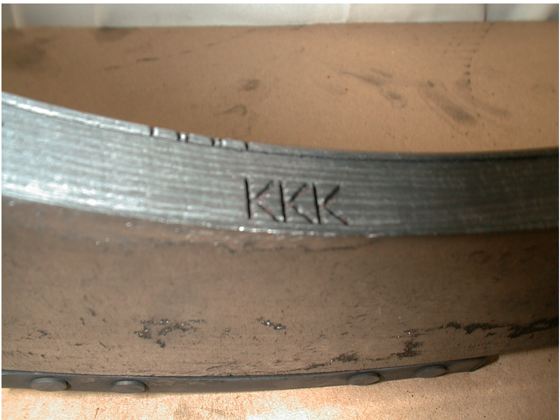
Rotor R2 - Unbalanced " 2 for 1" ( t_1=13\text{ mm} - t_2=2.5\text{ mm} )
