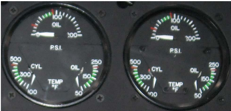
Figure 2. Correct configuration with Sigma Tek (Edo Aire) P/N 1U378-003-20, or P/N 1U378-003-20A
