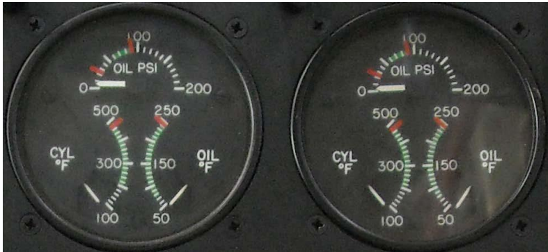
Figure 2. Correct configuration with Sigma Tek (Edo Aire) P/N 1U378-003-20, or P/N 1U378-003-20A
