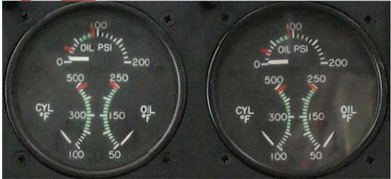
Figure 2. Correct configuration with Sigma Tek (Edo Aire) P/N 1U378-003-20, or P/N 1U378-003-20A
