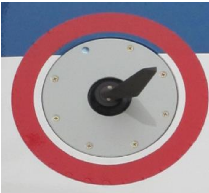
New AOA probe flat blanking plate cannot be customized
